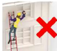
Incorrect – Overreaching and not maintaining three points of contact
